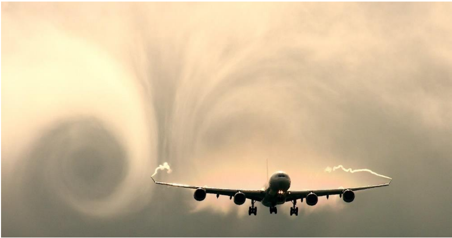
Figure 1. Wake vortex turbulence forming around an aircraft
